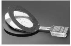
The ENVIRO-SEAL Type III Rupture Disc is also designed to burst in either the positive or vacuum direction at the same burst pressure. However, the ENVIRO-SEAL Type III Rupture Disc consists of two metallic top sections, one located on the process side and one on the vent side of the rupture disc. A single seal is located between the two top sections.
