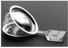
The CDCV Type Rupture Disc is the same design as the CDC Type Rupture Disc, with the addition of a vacuum support installed on the process side of the seal. This design provides process side corrosion protection and support for full vacuum conditions.
