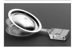
The CDC Type Rupture Disc is the basic Preformed Composite Rupture Disc design consisting of a slotted metallic top section and a fluoropolymer or metallic seal on the top section's process side. This basic design provides corrosion protection and excellent performance in low pressure applications where no backpressure or vacuum is expected.
