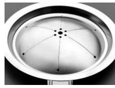
Continental's Preformed Composite Rupture Discs also feature our sevenhole pattern, positioned at the apex of the rupture disc's top section. This unique configuration, in combination with the pre-cut sections along the dome, provide non-fragmenting characteristics when used with a non-metallic or fluoropolymer seal. By using this sevenhole design, thicker, more durable materials can be used to manufacture the rupture disc while still achieving the high 80% operating-to-burst-pressure ratio.
