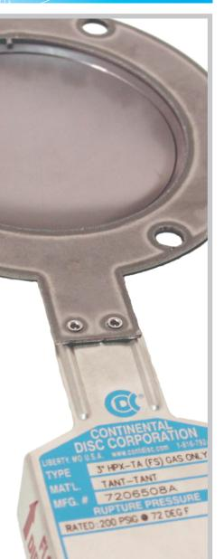
The HPX<sup>®</sup>-Ta Rupture Disc is a Tantalum semicircular scored reverse acting rupture disc designed specifically for use in highly corrosive media, such as bromine, chlorine, HCL, nitric acid or sulphuric acid. In certain concentrations, temperatures and moisture conditions, Tantalum is frequently the only suitable rupture disc material for the application.
