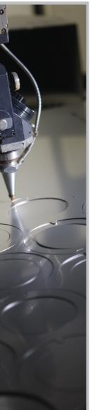
Continental Disc's solid metal, scored, reverse acting rupture discs are differential pressure relief devices that provide an instantaneous fully-open, non-reclosing design for protecting vessels, equipment and systems from an overpressure condition.
